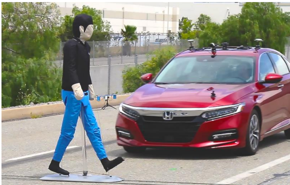
Rys. 2.9. Test systemu AEB PEDESTRIAN [14]
