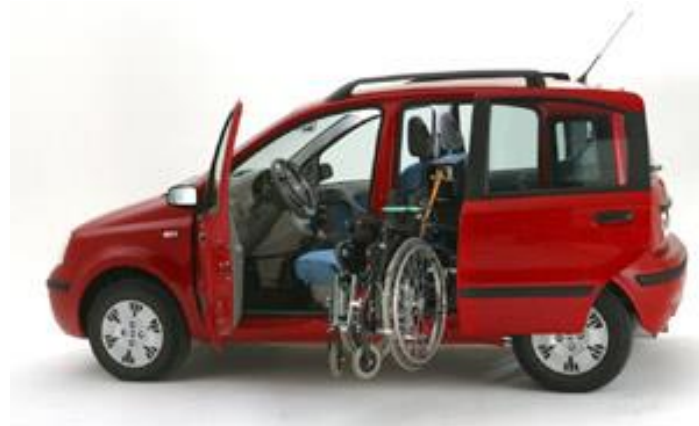
Figure 2. Wheelchair loading device [13]
