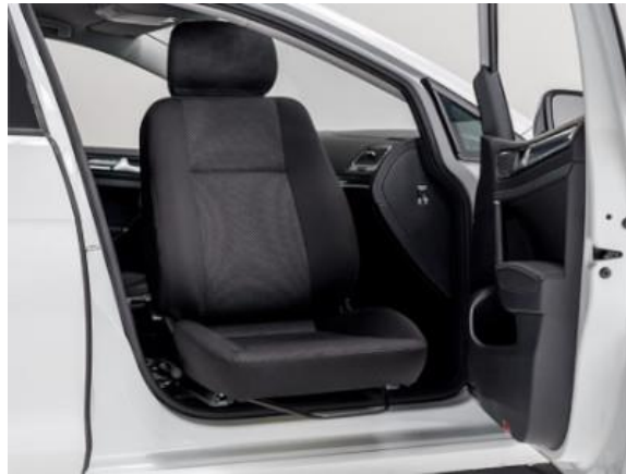
Figure 3. A rotatable seat facilitating boarding for disabled people [14]
