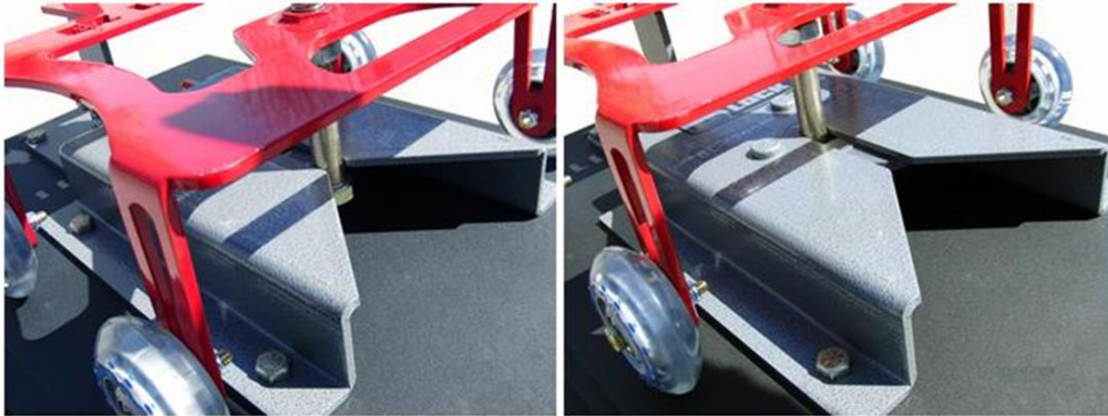
Figure 2. The EZ Lock Wheelchair Docking System [12].
