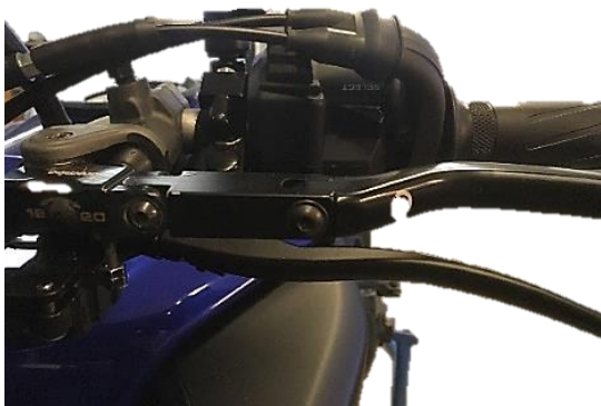
Figure 2. View of the left side of the steering wheel after relocating the right-hand controls (front view).
