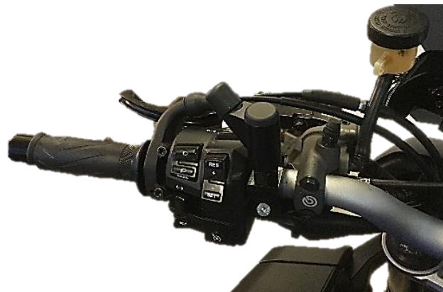
Figure 3. View of the left side of the steering wheel after relocating the right-hand controls (back view).
