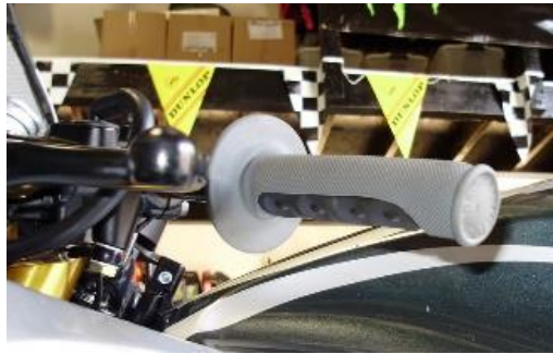
Figure 9. View of the pushbutton grips.
